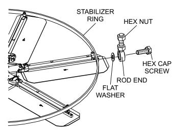
Figure 32. Stabilizer Ring Removal
